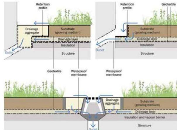
Drainage systems for an extensive green roof.
