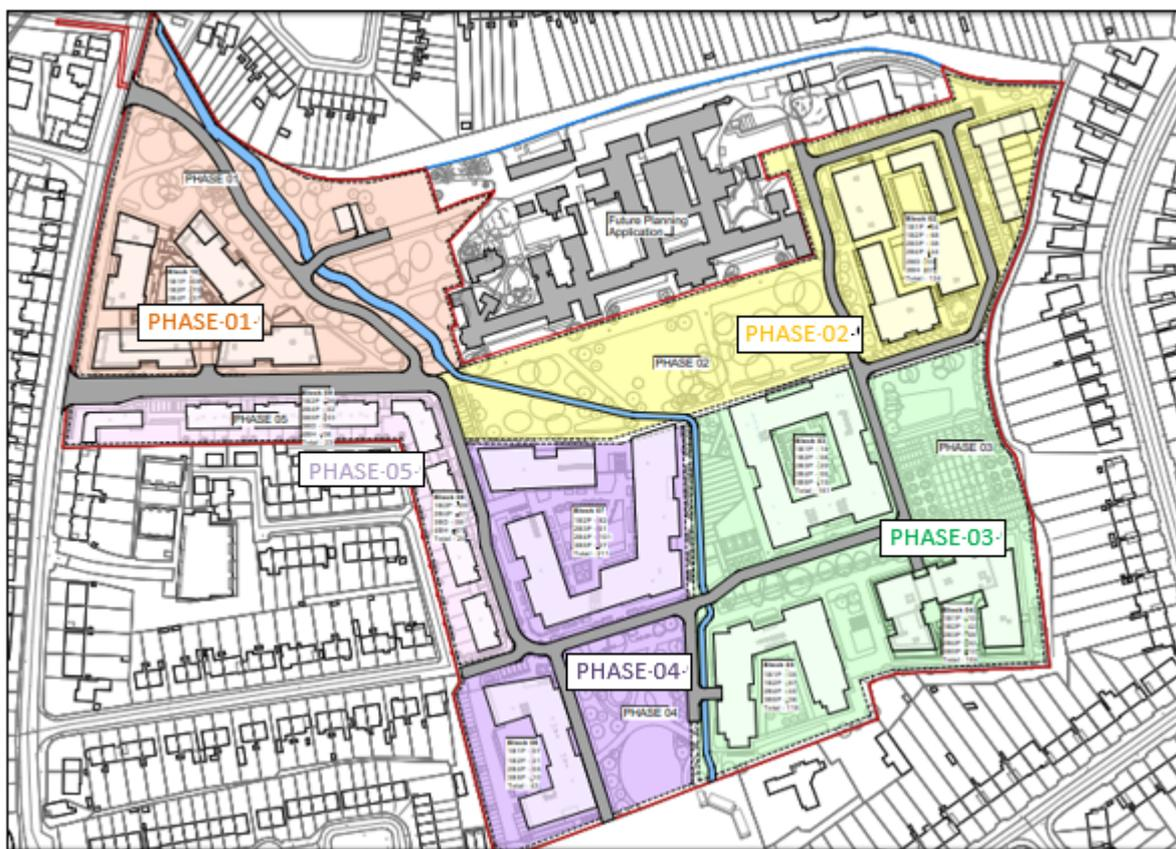
Figure 9.11 – Plan View of the Development Showing the Block Layout and Outline Phasing.
