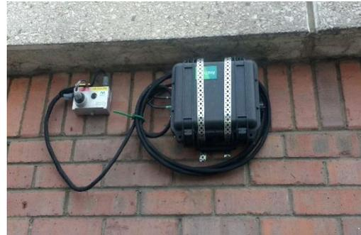
Photo 9.1: Typical Vibrograph installation
