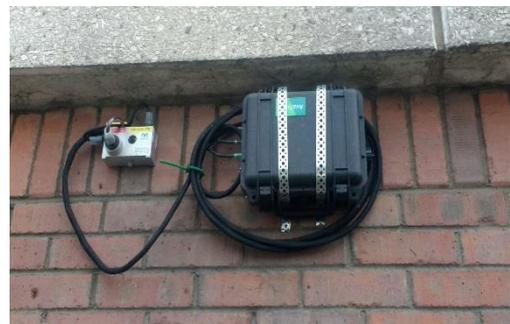
Photo 7: Typical Vibrograph installation
